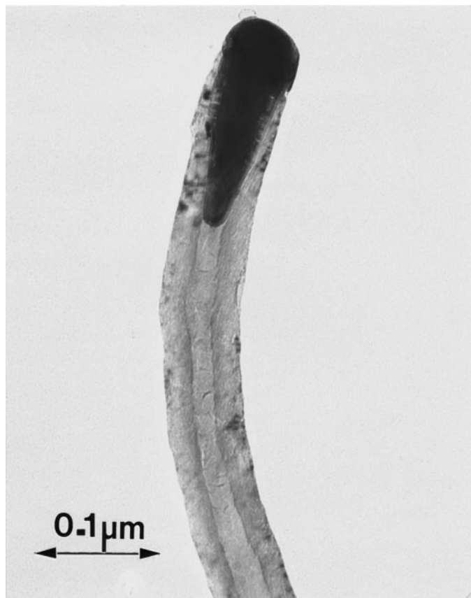
FIG. 11. Transmission electron micrograph showing the appearance of a "whisker-like" carbon filament produced from the interaction of an Fe-Ni (6 : 4) catalyst with C_2H_4/CO/H_2 (3 : 1 : 1) at 600°C.
